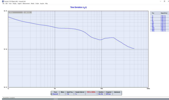
Fig. 4 TDEV of time transfer over the 166 km field fiber link
